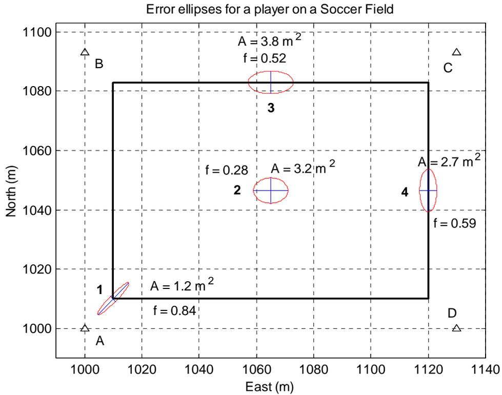
Figure 6. Area and flattening of error ellipses at four locations on a soccer field. Standard deviation of bearings  $1^\circ$ . Antennae at four corners  $A, B, C$  and  $D$ .
