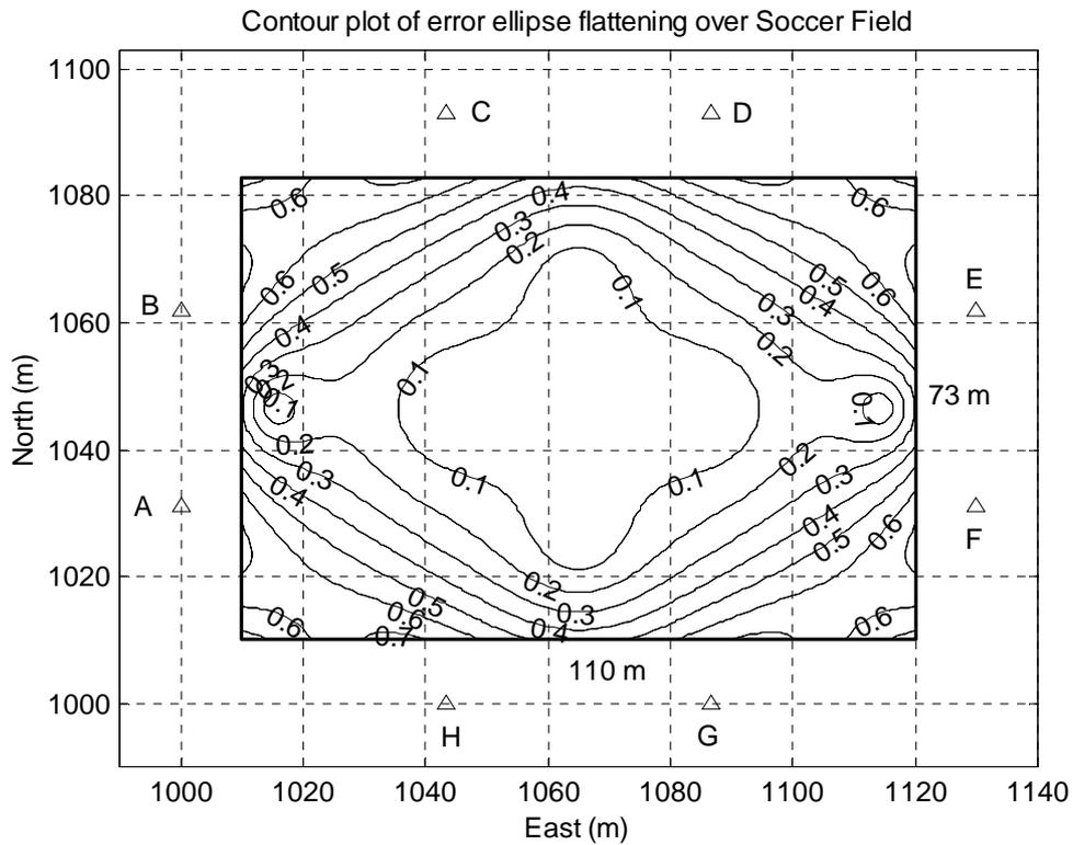
Figure 10. Contour plot of error ellipse flattening for computed positions over a soccer field. Standard deviation of bearings  $1^\circ$ . Antennae in pairs along four sides.
