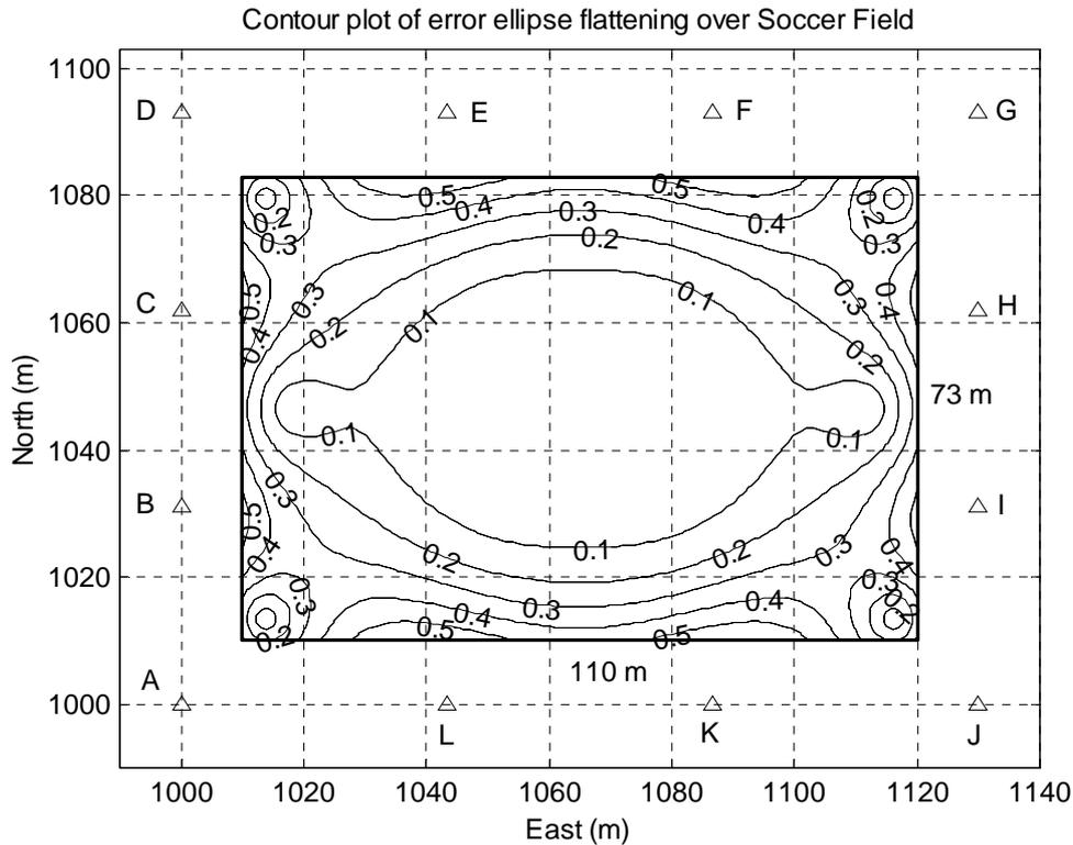
Figure 11. Contour plot of error ellipse flattening for computed positions over a soccer field. Standard deviation of bearings  $1^\circ$ . Twelve antennae in pairs along four sides and at the corners.
