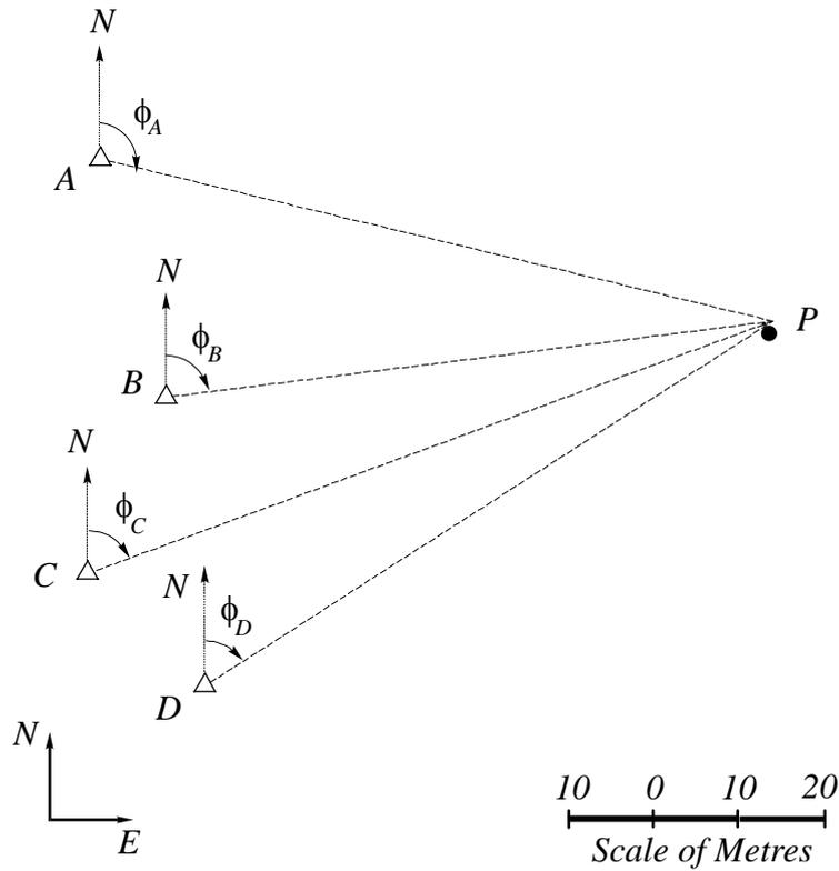
Figure 3. Athlete at *P* and bearings from antennae locations *A*, *B*, *C* and *D*.
