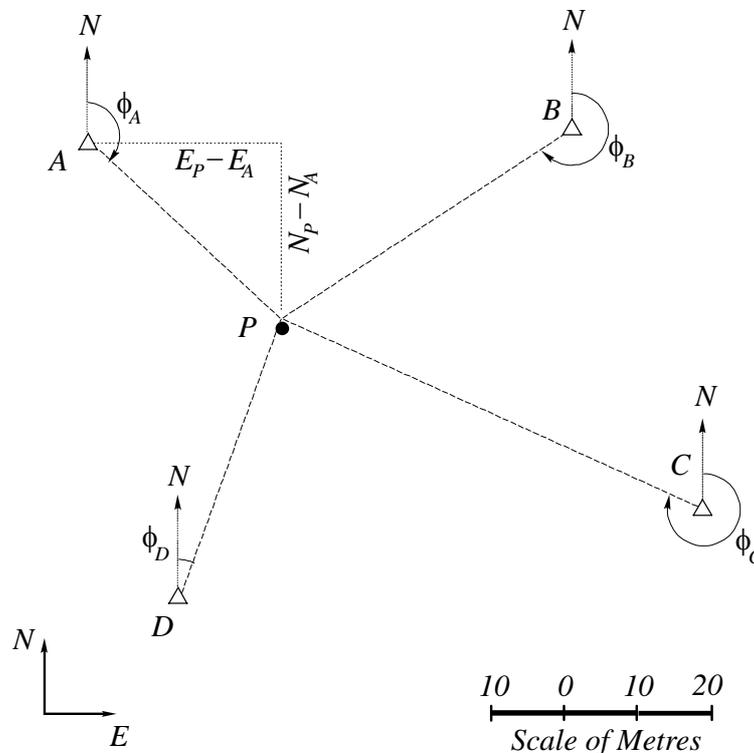
Figure 1. Athlete at  $P$  and bearings from antennae locations  $A$ ,  $B$ ,  $C$  and  $D$
