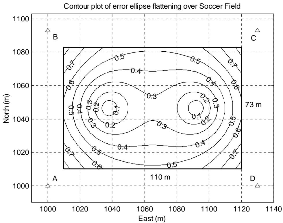
Figure 7. Contour plot of error ellipse flattening for computed positions over a soccer field. Standard deviation of bearings  $1^\circ$ . Antennae at four corners A, B, C and D.
