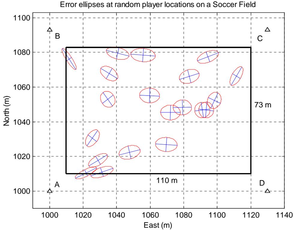
Figure 5. Error ellipses at random locations of a player on a soccer field. Standard deviation of bearings  $1^\circ$ . Antennae at *A, B, C* and *D*.
