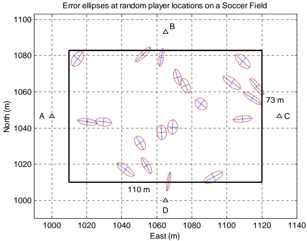
Figure 8. Error ellipses at random locations of a player on a soccer field. Standard deviation of bearings  $1^\circ$ . Antennae on four sides.
