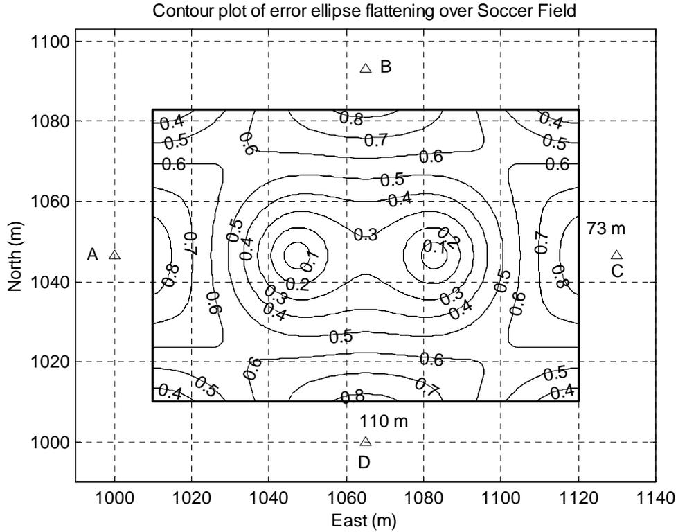
Figure 9. Contour plot of error ellipse flattening for computed positions over a soccer field. Standard deviation of bearings  $1^\circ$ . Antennae at four sides A, B, C and D.
